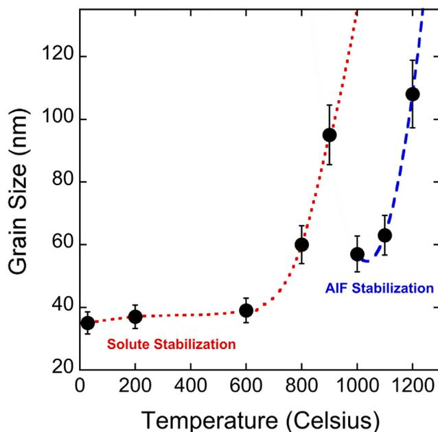
**Fig. 4.** XRD grain size analysis of the Ni-6 at.% W electrodeposited alloys after annealing for 1 h at different temperatures. The data shows two distinct regions of stabilization by solute segregation and AIF formation. Rough trend lines are added to guide the eye and highlight these two regions.
