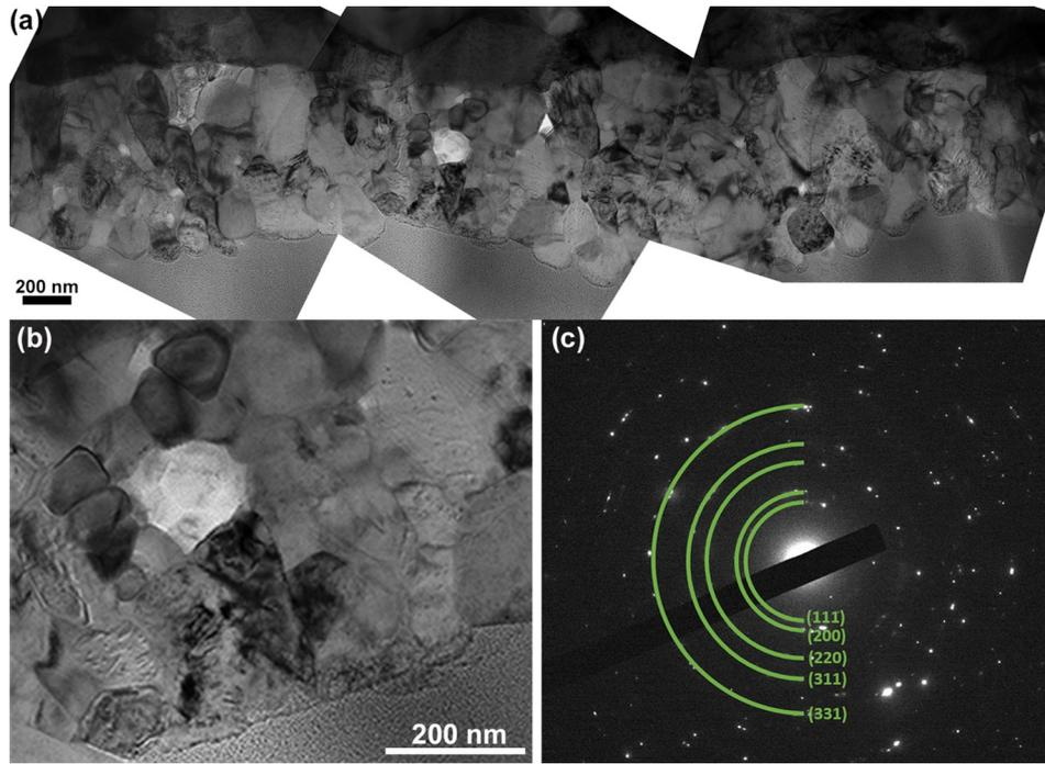
**Fig. 1.** Bright field TEM images of nanocrystalline Ni-5 at.% W after a 24 h anneal at 650 °C and then a 10 min anneal at 1100 °C. (a) shows the overall film microstructure, while (b) shows a magnified image where equiaxed grains are observed. (c) The selected area electron diffraction pattern shows that only face centered cubic (fcc) Ni rings are present.
