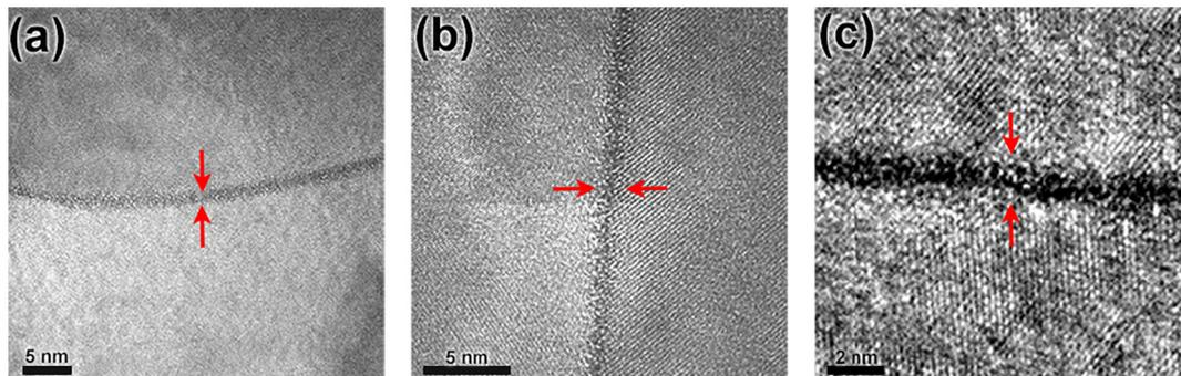
**Fig. 2.** High resolution TEM images of ~1 nm thick amorphous intergranular films in the Ni-5 at.% W alloy after quenching from 1100 °C, with multiple examples shown in (a)–(c).
